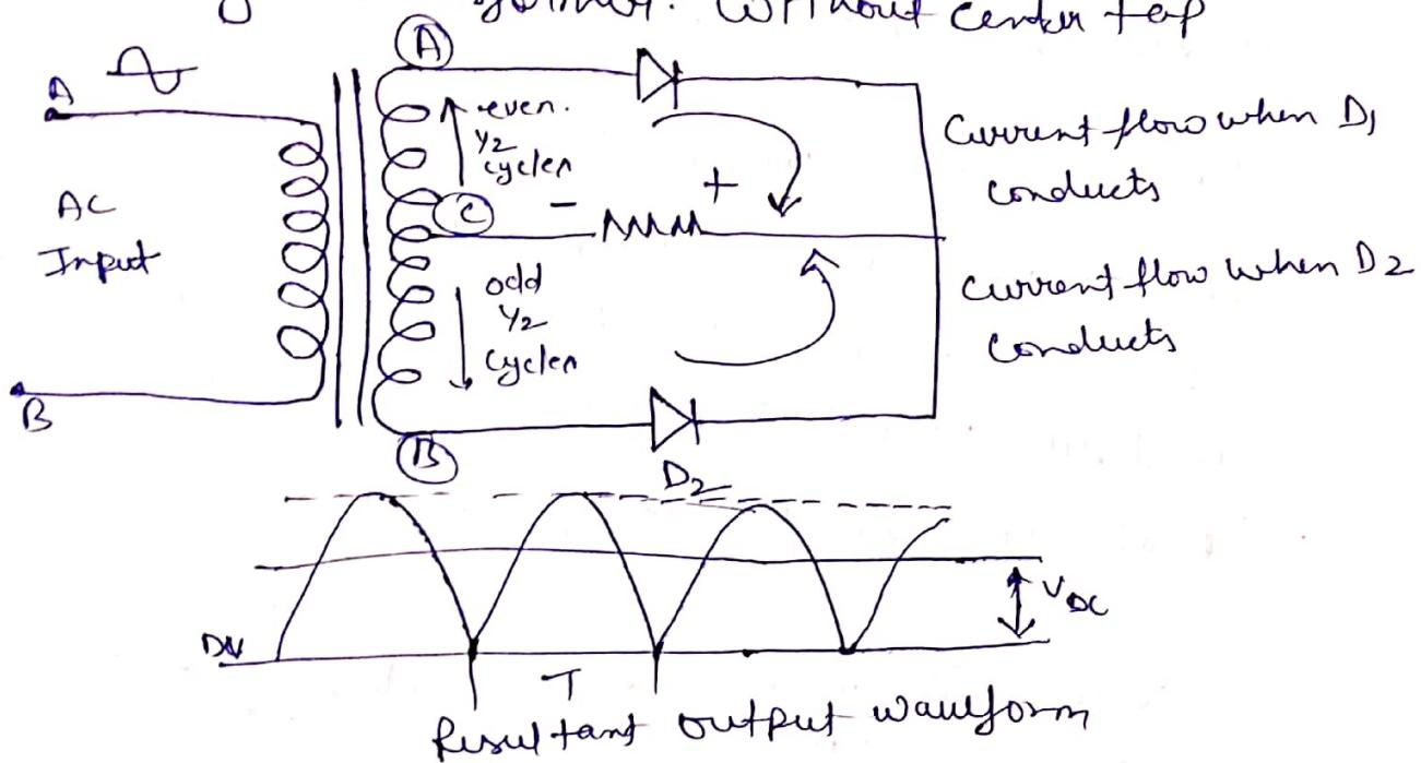
The full wave rectifier circuit consists of two half-wave diodes connected to a single load resistance ( $R_L$ ) with each diode taking turns to supply current to the load. When point A is positive with respect to point C, diode D<sub>1</sub> conducts in the forward direction as indicated by the arrow. When point B is positive (more negative) than point A, diode D<sub>2</sub> conducts in the forward direction.
