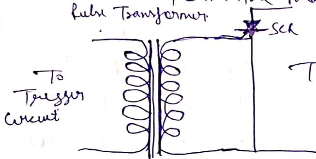
only one half of the cycle is available for the gate drive to control the firing angle and next half of the cycle a reverse voltage is applied between the gate and cathode.
