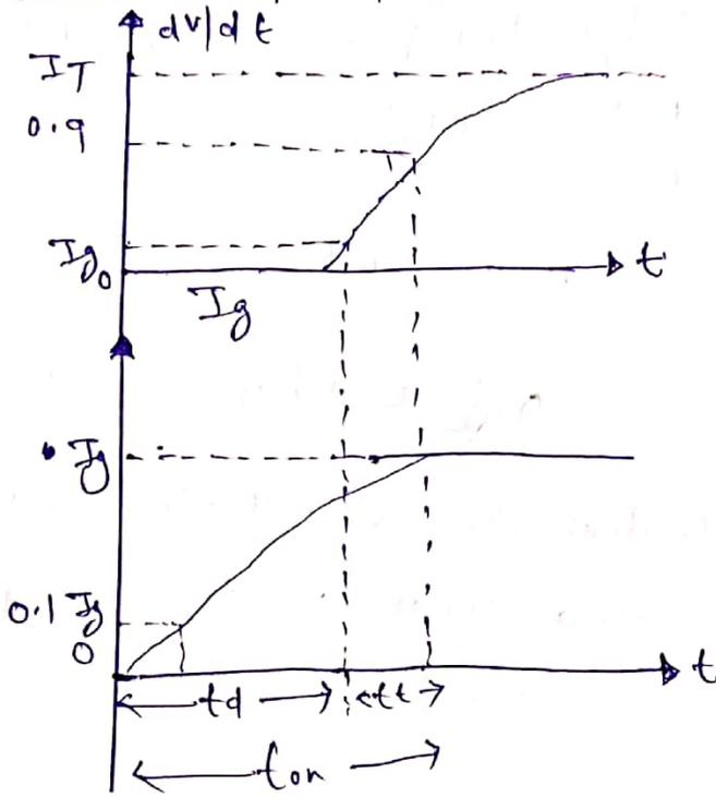
When the thyristor is forward and a gate signal is injected by applying positive gate voltage is applied between cathode and terminals then the thyristor turned on.
