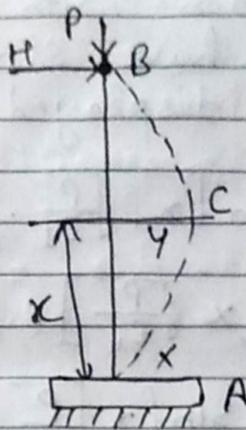
As we know that for long column, when one end of the column is fixed and other end is hinged, we will have following condition as mentioned here.
