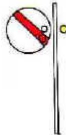
(b) Disc type Shunt signal in Multiple-Aspect Signalling Territory “On” Position “Off” Position
