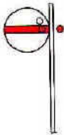
(b) Disc type Shunt signal in Multiple-Aspect Signalling Territory “On” Position “Off” Position
