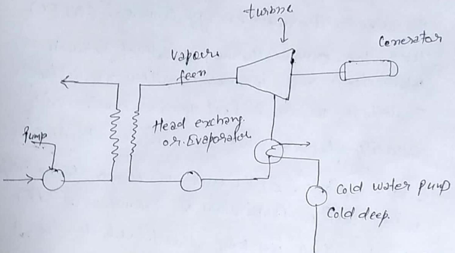
In this system, the warm water from ocean surface is admitted through the decelerator to the flash evaporator which is maintained under high vacuum. As a result a low pressure stream is generated due to throttling effect and the remainder liquid is discharged back to the ocean at right depth, the decelerator also removed. The dissolved non-condensable gases from water before supplied to the evaporator.
