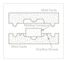
Molding compound is placed in an open, heated mold cavity.
