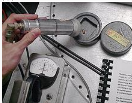
Laboratory use of a G-M counter with end window probe to measure beta radiation from a radioactive source
