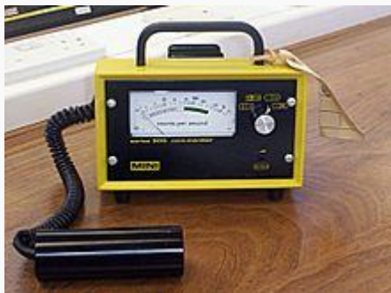
A "two-piece" bench type Geiger–Müller counter with end-window detector.
