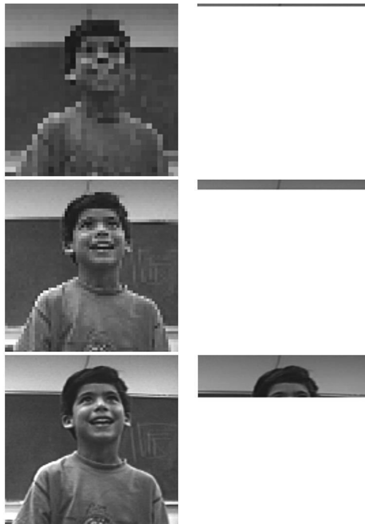
FIGURE 7.4 Comparison between the received image using progressive transmission and using the standard raster scan order.
