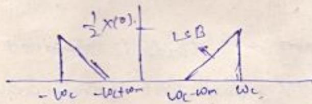
SSB-SC wave with single tone modulating signal  $\Rightarrow$
