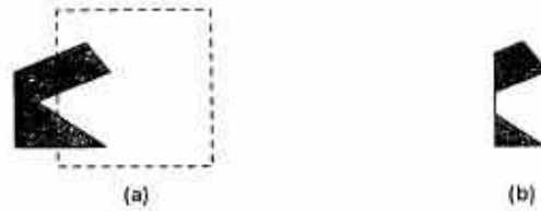
Fig. 5.27 Clipping the can cave polygon in (a) with the Sutherland-Hodgeman algorithm produces the two connected areas in (b)
