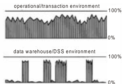
Figure 7.2. The Fundamentally Different Patterns of Hardware Utilization between the Data Warehouse Environment and the Operational Environment
