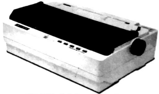
Fig. 2.29. A Daisy wheel printer
