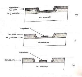
silicon integrated circuits. Undoped polysilicon has relatively high resistivity. The resistivity of polysilicon can be reduced, however, by doping it with impurity atoms. After deposition, the polysilicon layer is patterned and etched to form the interconnects and the MOS transistor gates
